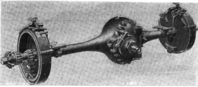
Rear Axle in One Piece of Drawn Steel.
